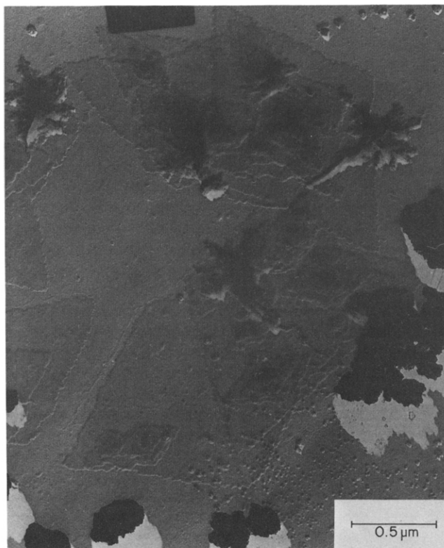
Figure 9 Electron micrograph of single step crystallization sample, T_c = 86.2^\circ\text{C} , showing single crystal lamellae and sphere-like structures
